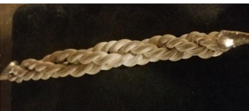
The ends are then worked out in a similar fashion to the wires. The bracelet is then formed to shape, then polished.
