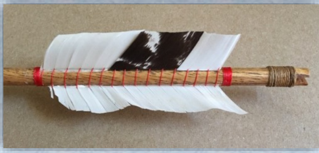
Photo 4: Spliced fletching using partial length fletches
