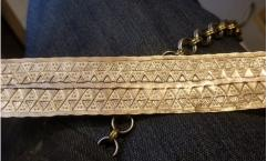
stamped, followed by shaping it by either tapping it out from the inside with a round peening hammer with a softer backing (to not mar up the stamping), or fixing a round peening surface to brace the inside, and tapping the outside with a rawhide mallet (likely both).
